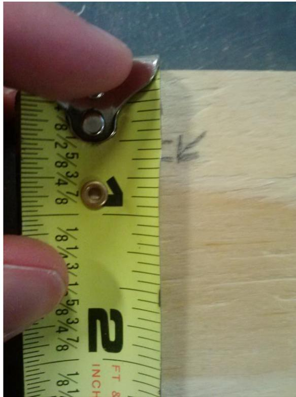
6. Apply drill press, followed by hammer. Your hole should likely be  $1/4$ " in diameter to match the rod. This makes a fit which is snug enough to keep the rod from going anywhere, especially as there is no sideways force on it during operation.
