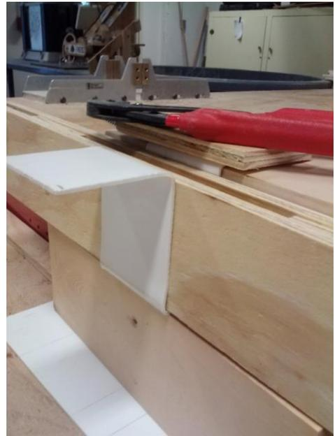
15. Position everything on the board. Possibly trace positions so things don't move. Drill through the PVC pieces (3/16" bit, I think) and bolt them down. Wood glue the motor mount down. Remember: Your motor mount is going to go beside the arm so the motor sticks over it. Needless to say, in no way attach the arm itself to the board.
