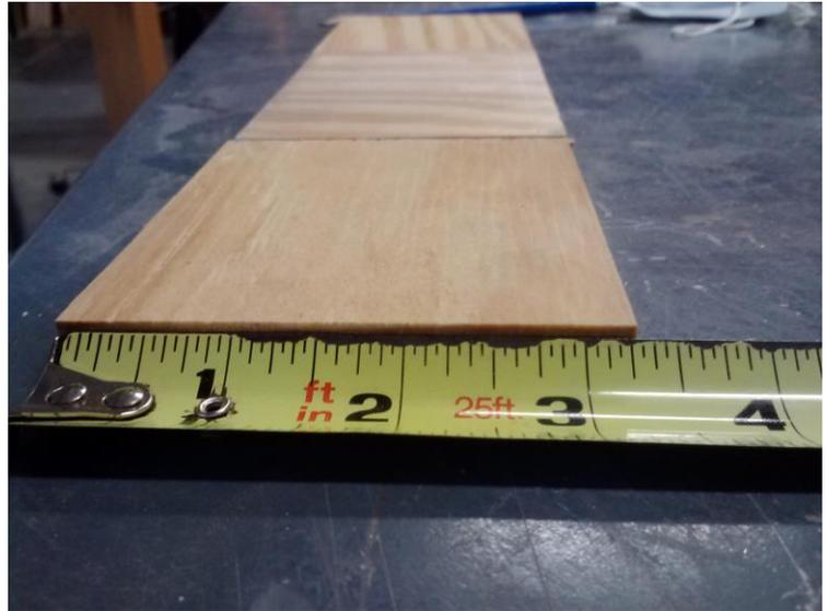
9. Take your "one by four" which is really 3/4" thick and cut off 2 rectangular prisms which are 3/4" x 3/4" x 3 1/4". These will brace your motor platform. Wood glue them to the tops of the side pieces of the motor mount (the 4" long ones). Don't forget the clamps. Pictured is one of my friends, the narwhals.
